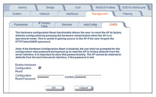
Figure 4-22 Hardware Configuration Reset
